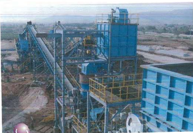
A view of the MSPL Exports plant showing Hopper, Crushers and Conveyor system.
